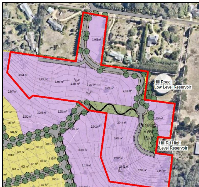
Figure 18: Lots to be connected to Hill Rd High Level Zone (Source: UWS, August 2020, Figure 4-1)
